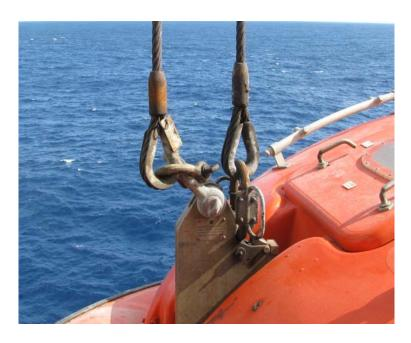
c The forward lifting ring became disengaged because it slipped between the lifting hook and the locking mechanism.
