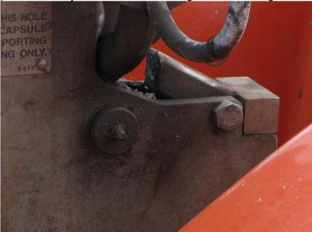
i. We observed that in certain circumstances the locking mechanism can stay in the open position, permitting the lifting ring to slip out.
