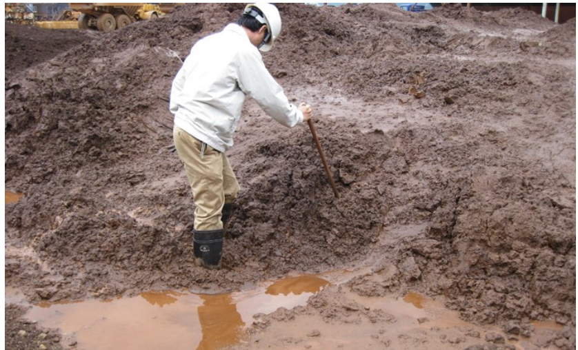
Typical appearance of zinc concentrate presented for loading in Bar, Montenegro
