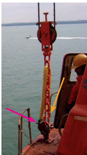
An on-load release hook with FPD attached at hanging-off lug (magenta arrowed).
