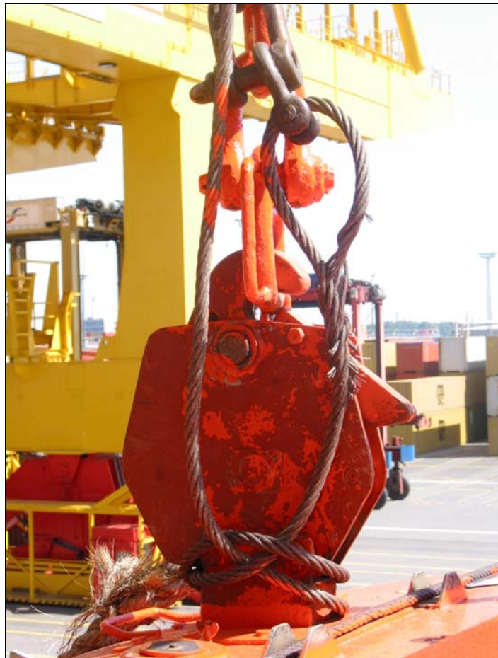
Figure 8: Front releasing hook on the starboard lifeboat with securing cable
