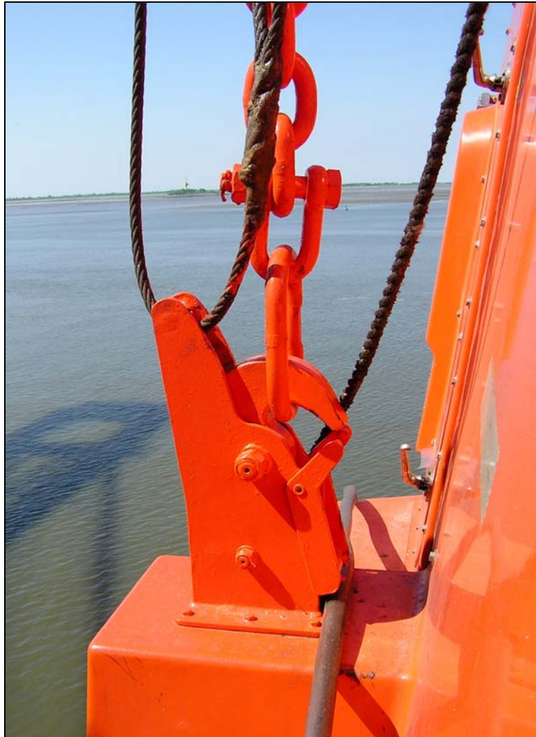
Figure 19: Aft releasing hook on the new port lifeboat, marking no longer visible
