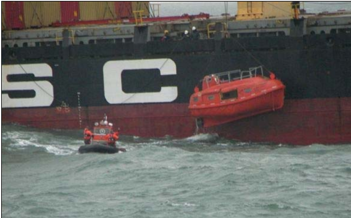
Figure 3: Taking the lifeboat onboard using the MSC GRACE cargo gear and a Federal Police control boat
