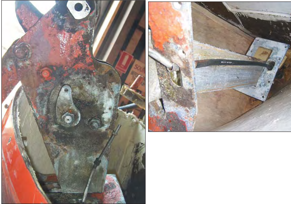
Figures 14: Forward hook, forward hook attached at keel block
