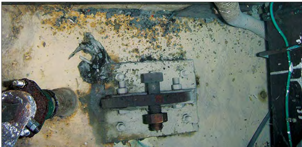
Figure 15: Port lifeboat after hook keel attachment
