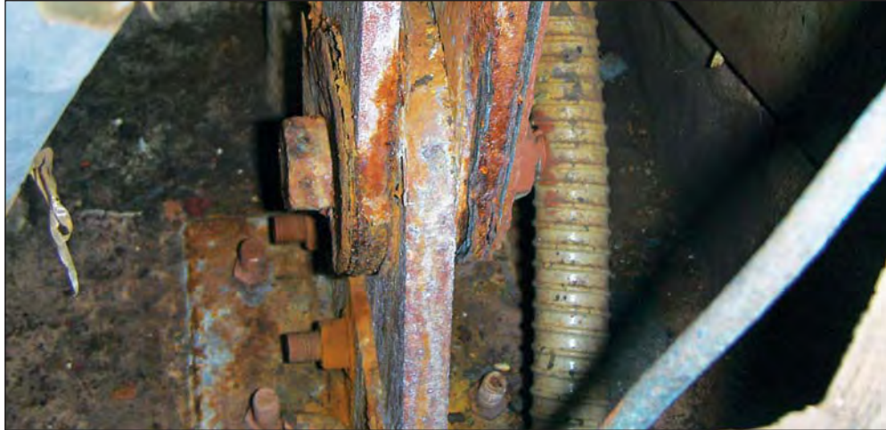
Figure 17: Starboard lifeboat after hook keel attachment
