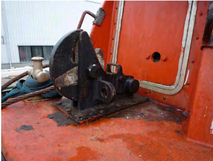
Photo 8: Hook as fitted. Note lug on side of side plate. There is another on the opposite side.
