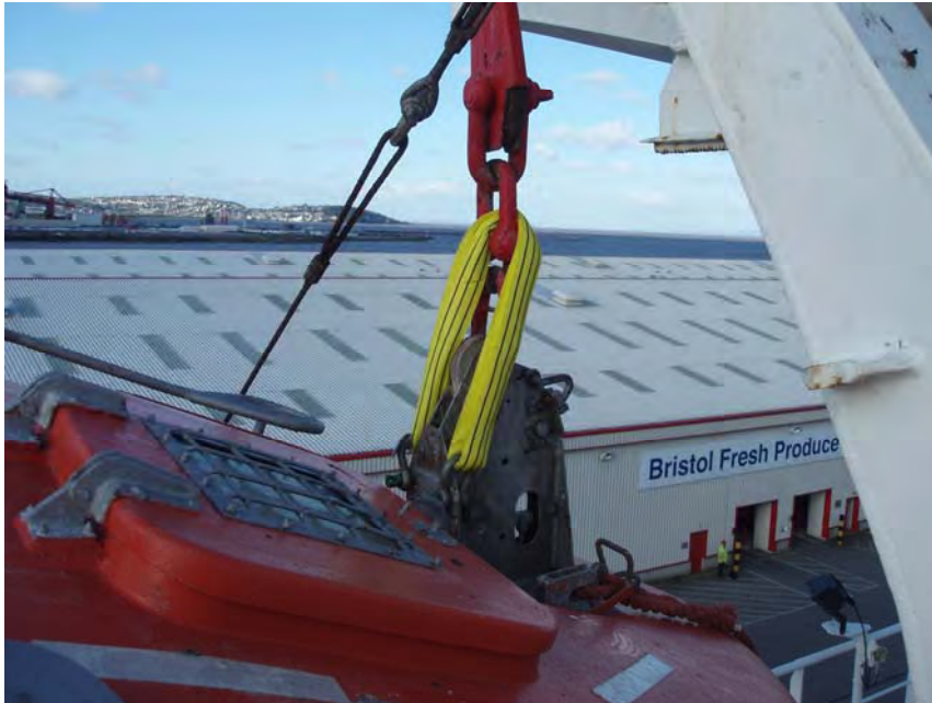
Continuous sling in place over-riding on-load release
