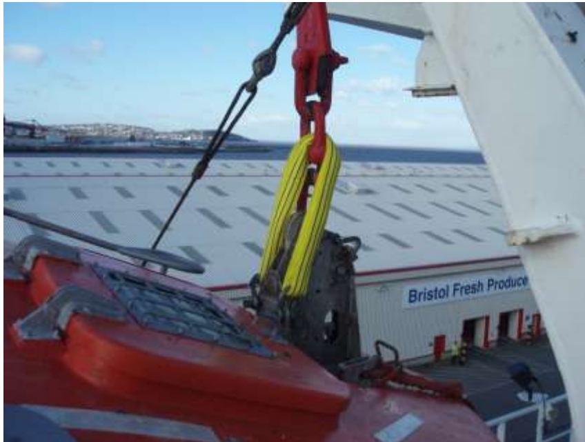
Continuous sling in place over-riding on-load release
