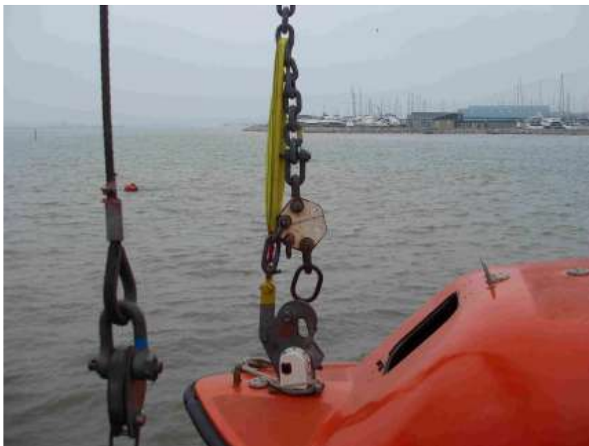
FPD taking load during exercise, simulating premature release of on-load hook. Note boat is not waterborne but suspended just above the water – a safety precaution for avoiding injury to personnel or damage to structures during the exercise.
