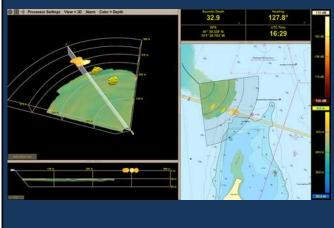
Forward-Looking Sonar system- Located on the bulb it detects objects in the water column up to 500 meters ahead and a range of 90° up/down.
