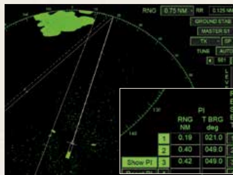
Use of index lines for position monitoring and course alteration
