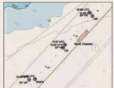
Position fixing using LOPs with DR or EP navigation on ECDIS
