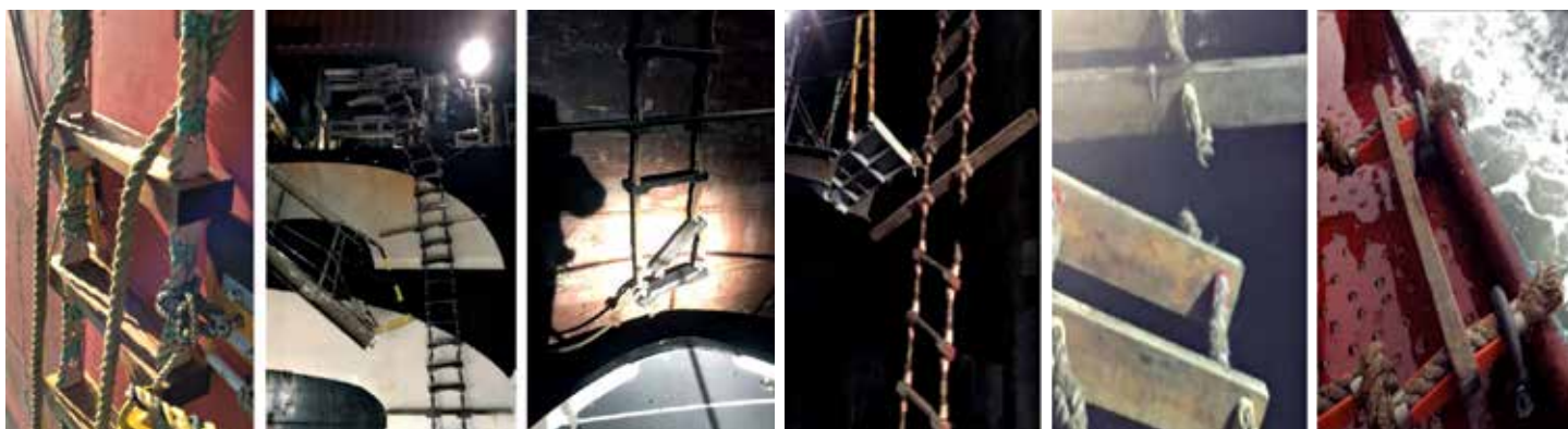
There are many ways that a pilot ladder can be unsafe – would you want to climb any of these?
