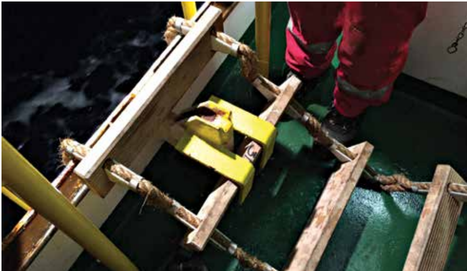
An incorrectly secured ladder and uneven steps - just two examples of bad practice to avoid
