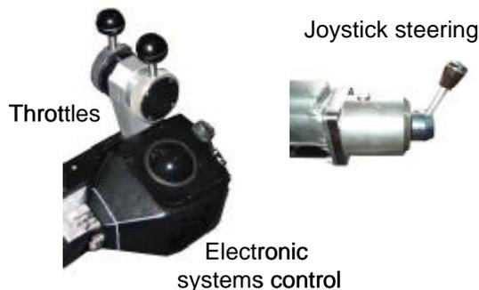
Figure 8: Arm mounted controls
