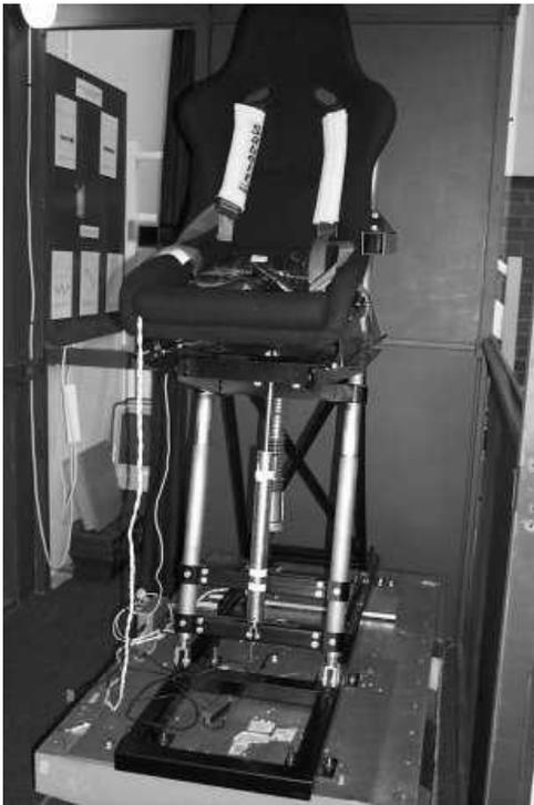
Figure 6: New seat undergoing hydraulic platform tests
