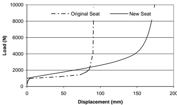
Figure 2: Typical spring characteristic
