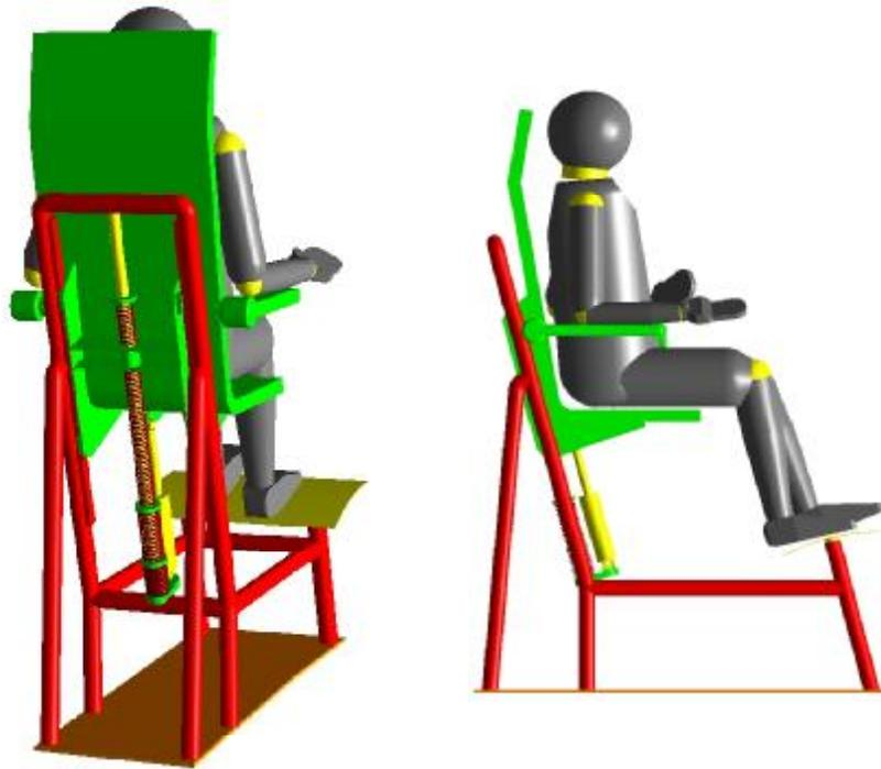
Figure 4: New seat concept design
