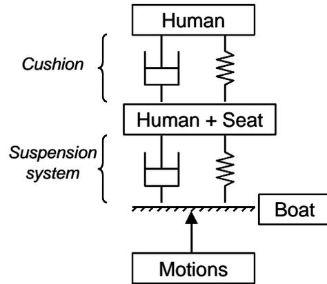
Figure 1: Generic seat suspension system model
