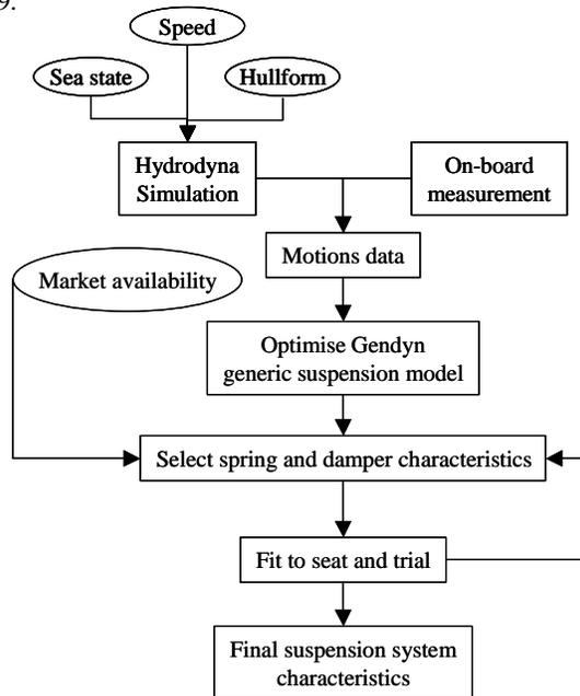
Figure 9: Tailored seat suspension system methodology
