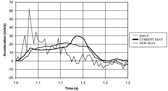
Figure 3: Response of seat models to a  $62\text{m/s}^2$  input
