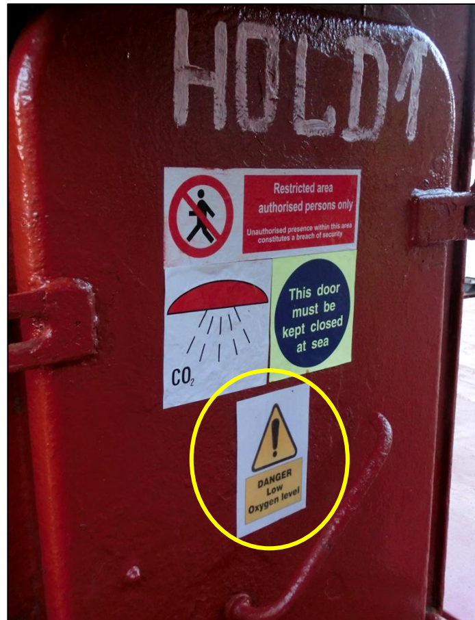
Figure 12: Warning sign affixed to the cargo hold access door
